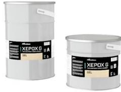
Two-components epoxy gel adhesive for structural usage, applicable via trowel also on vertical surfaces, permits the realization of thick or uneven layers. Suitable for large timber overlaps, for gluing structural reinforcing elements by using glass or carbon fiber textures and for metal or timber coatings. Spreadable. Shelf life 36 months in the original unopened packaging, at temperatures between +5°C and +30°C.
