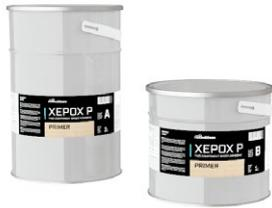
Two-component epoxy adhesive with extremely low viscosity and high wetting properties for structural reinforcements through carbon or glass fiber textures. Useful to protect sanded metal sheets SA2,5/SA3 (ISO 8501) and to realize FRP (Fiber Reinforced Polymers) bits. Applicable by roller, spray and brush. Shelf life 36 months in the original unopened packaging, at temperatures between +5°C and +30°C.
