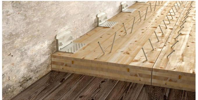
3 Floor reinforced with LBB perforated strap
