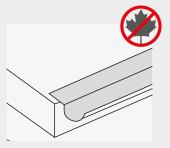
Check that the gutter and ridge are free of obstacles that could impede air circulation.
