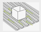
Avoid battening or other impediments that could block the upward flow of air heated along the slope.
